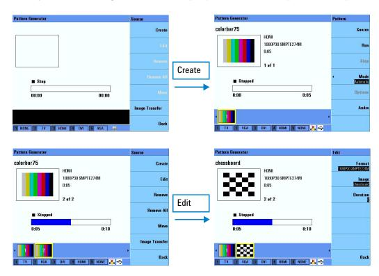
Figure 3-2 Inserting steps in a particular sequence
