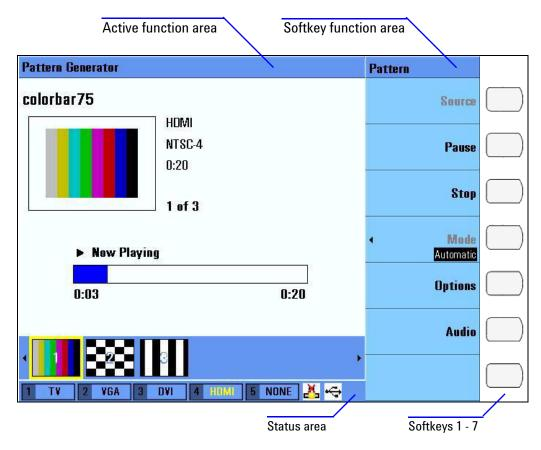
Figure 2-10 Front panel LCD display
