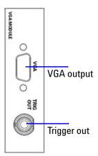
Figure 6-2 Analog RGB card (VGA card) rear panel
