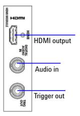
Figure 6-4 HDMI 1.2 generator card rear panel
