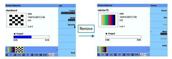
Figure 3-3 Removing steps in a particular sequence
