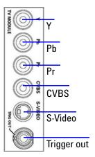
Figure 6-1 Analog TV card rear panel
