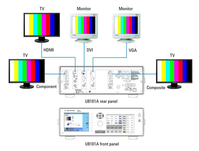
Figure 3-4 Simultaneous test setup example
