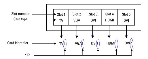
Figure 7-2 Card configuration for Example 1
